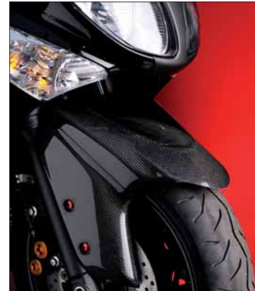
PARAFANGO ANTERIORE / front mudguard
